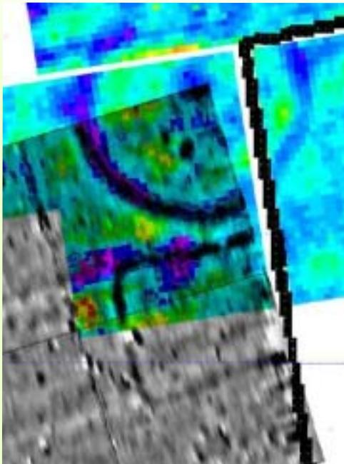
A double overlay showing in colour a **resistivity** survey of a local tumulus site. Overlaying, in greyscale, is a **magnetometry** survey revealing a portion of a rectangular enclosure as yet to be identified. The modern field boundary shows as a thick dark line.
